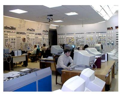
Full-scope and analytical simulators provide needed training for operators at Soviet-designed nuclear power plants. U.S. and Russian contractors are working together to design simulators to replicate the configuration and behavior of specific reactors in Russia and Ukraine.
